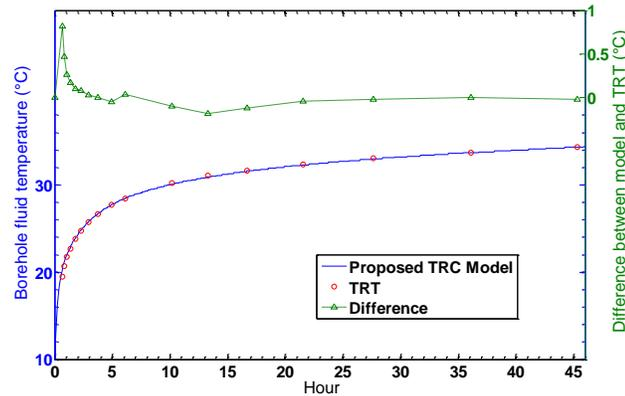
Figure 3 Results of the TRT and of the simulation with the proposed TRC model
