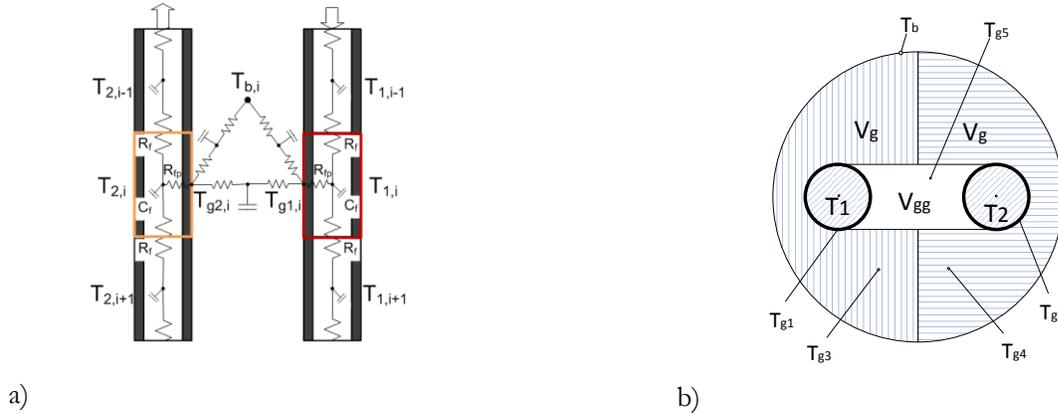
**Figure 1** Axial and radial representation of the various nodes in the TRC model proposed by Godefroy (2014)
